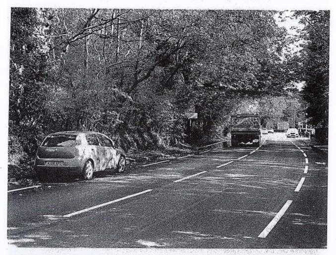
2. Photo showing dilapidated traffic island causing pinch point and gap in markings
